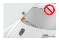
Make sure that the wiper is stopped near the upper reverse position.
