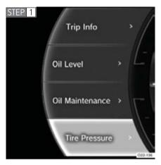
Select "Tire Pressure" and press right on the control pad.
