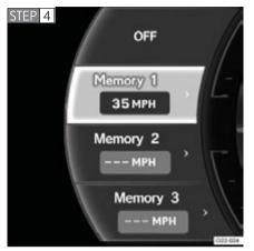
Press left on the control pad to enter the desired speed.
