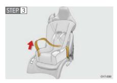
Fully extend the lap belt and allow it to retract to put it in lock mode. In lock mode, the belt cannot be extended.
