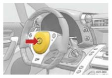
To sound the horn, press the pad in the middle of the steering wheel.
