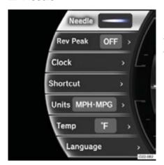
Each time right on the control pad is pressed, the color of the tachometer needle will change as follows:
