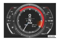
To help protect the engine, the red zone of the tachometer starts at different engine speeds ranging from 4400 rpm to 9000 rpm depending on the engine coolant temperature.
