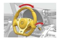
When starting the engine, the ignition switch may seem stuck in the "LOCK" position. To free it, turn the key while turning the steering wheel slightly left and right.
