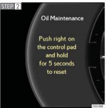
Press and hold right on the control pad for 5 seconds.
