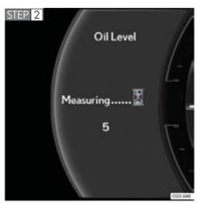
The amount of engine oil remaining is measured automatically.
