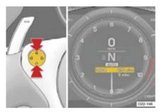
The information on the trip information display can be changed when in the normal display by pressing up or down on the control pad.
