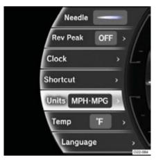
Each time right on the control pad is pressed, the distance (miles, km), the speed (MPH, km/h) and the fuel consumption (MPG, km/l, L/100km) measurement units will be changed.
