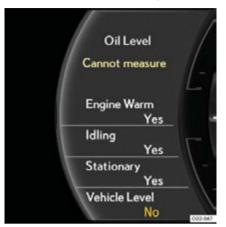
If measurement cannot be performed, the item with "No" displayed may be the cause. Check the following items and then attempt to perform the measurement again:
