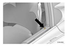
The indicator light flashes after the key has been removed from the ignition switch to indicate that the system is operating.
