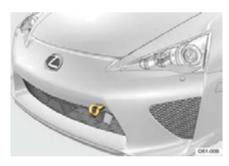
If a flatbed truck is not available, in an emergency your vehicle may be temporarily towed using a cable or chain secured to the emergency towing eyelet. This should only be attempted on hard, surfaced roads for short distances at low speeds. A driver must be in the vehicle to
