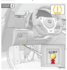
Press and hold the tire pressure warning reset switch until the tire pressure warning light flashes slowly 3 times.
