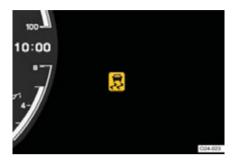
The slip indicator flashes to indicate that the ABS/VSC/TRAC/hill-start assist control systems are operating.
