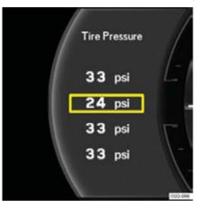
If a tire is insufficiently inflated, an amber frame will be shown.
