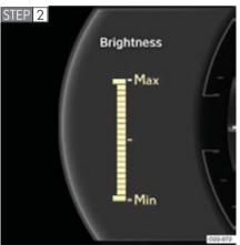
Adjust the brightness by pressing up and down on the control pad.
