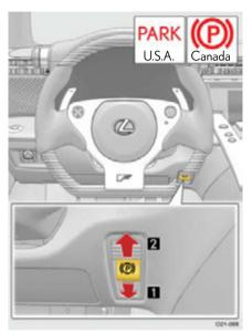
Press the switch to set the parking brake.
