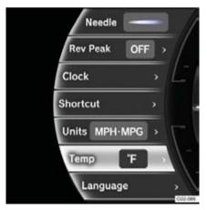
Each time right on the control pad is pressed, the temperature display unit will be changed (Fahrenheit, Celsius).
