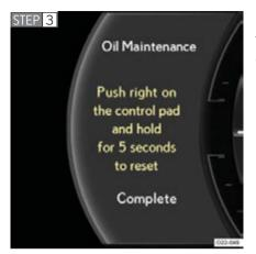
"Complete" will be displayed when the reset procedure has been completed.
