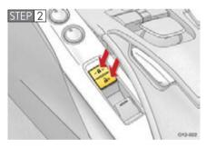
Check that Neutral is selected  $(\rightarrow P. 103)$ , press and hold the door lock switch (  $\bigcirc$  or  $\bigcirc$  ) for about 5 seconds then release.
