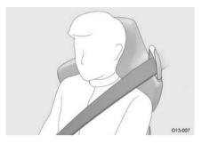
When fastening the seat belt, always ensure that it passes through the seat belt guide.
