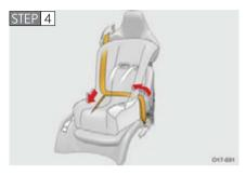
While pushing the child restraint system into the seat, allow the lap belt to retract until the child restraint system is securely in place.
