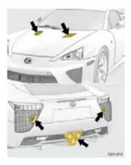
Do not touch the hood grilles, bezels in the radiator grilles, or exhaust pipes and surrounding area while the engine is running or immediately after turning the engine off. Doing so may cause burns.
