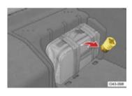
An exclusive hub socket for the wheel bolts of the LFA is contained in the tool bag. A 1/2inch (12.7 mm) drive extension bar and a torque wrench are required to tighten the bolts.
