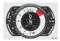
When the engine speed reaches or exceeds 6000 rpm, an afterimage of the tachometer needle will be displayed at the highest engine speed for approximately 0.5 seconds.
