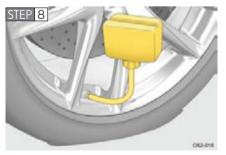
Inject the sealant that is in the bottle. Hold and tilt the bottle, then squeeze sealant out of the bottle as shown.
